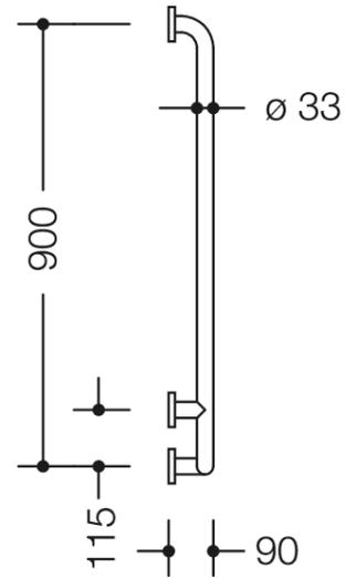
Abmessungen in mm
